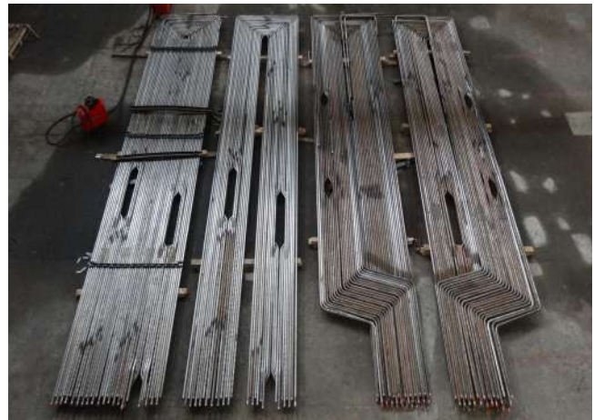
Have a seat production experience complete screen panels, including membrane panels using various spacing parts and stud-attack-wire-melting-wear-resistant layer
