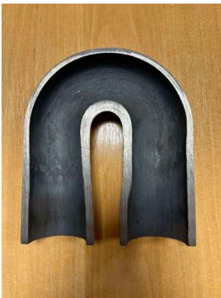
Steeply curved bend with radius bending up to 0.65D
