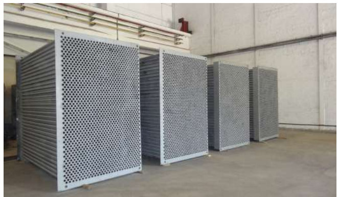
Tubular air preheater boiler with a capacity of 900 tons of steam time
